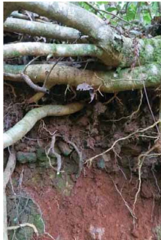
Figure 3.6 Close up of soil creep. A thin layer of soil and organic matter overlying a layer of rocks over thin soil over strongly weathered basalt
